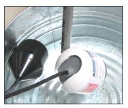
When the float reaches the appropriate angle it will trigger the switch and you will know whether the float is working properly.
