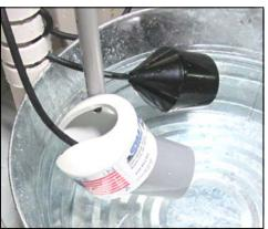
Then slide the float check over the float. While lifting the float apply torque to the handle so that you are pulling the float away from the float holder. This will hold the float in the float check.
