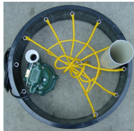
Picture of 4 legs disconnected on 24" riser. Small pump & 4" pipe for size reference.
