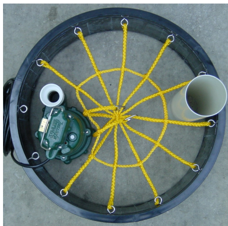
Picture of 2 legs disconnected on 24" riser. Small pump & 4" pipe for size reference.
